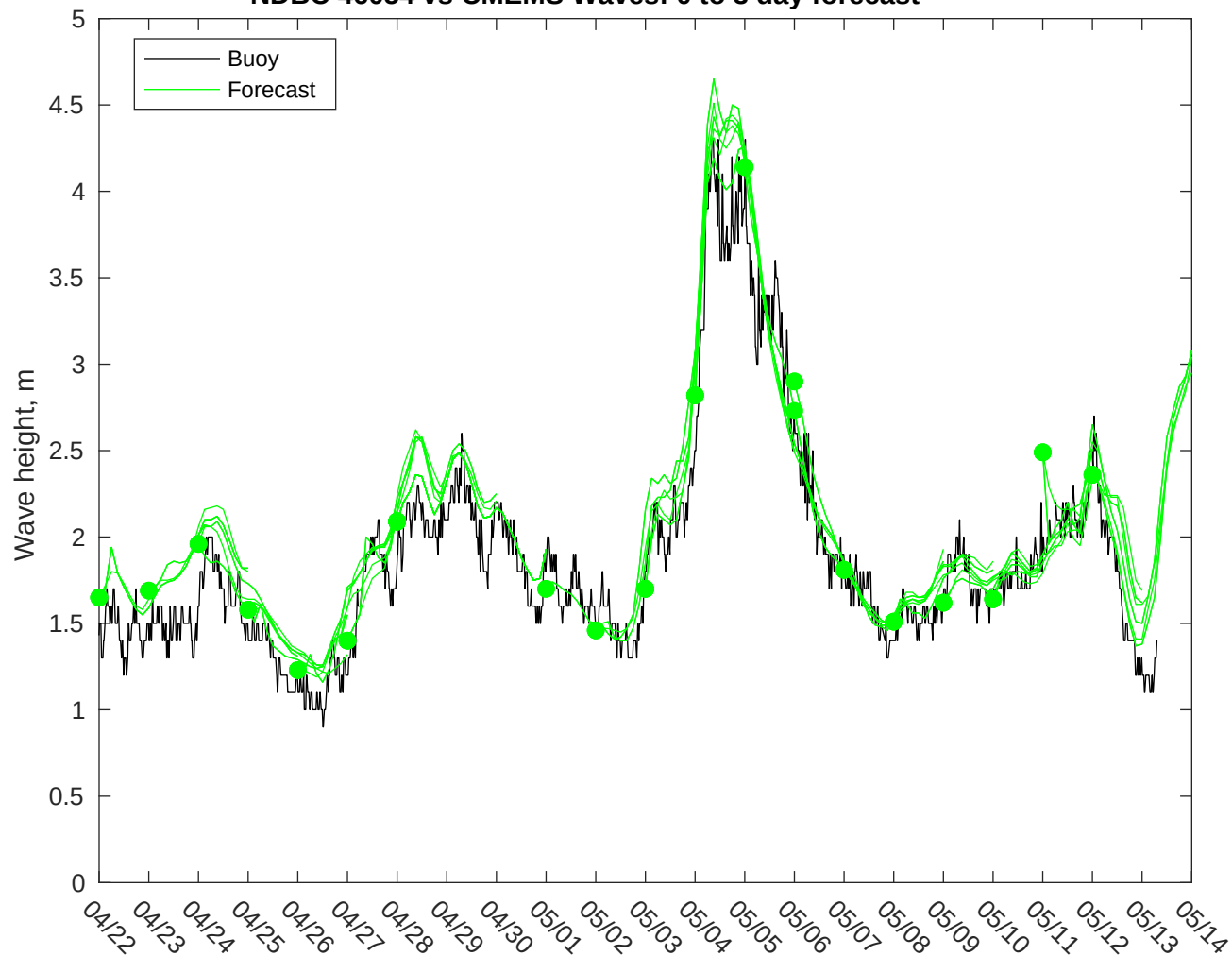
NDBC 46054 vs CMEMS Waves: 0 to 3 day forecast
