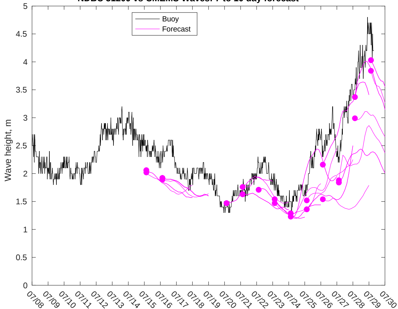
NDBC 51209 vs CMEMS Waves: 7 to 10 day forecast
