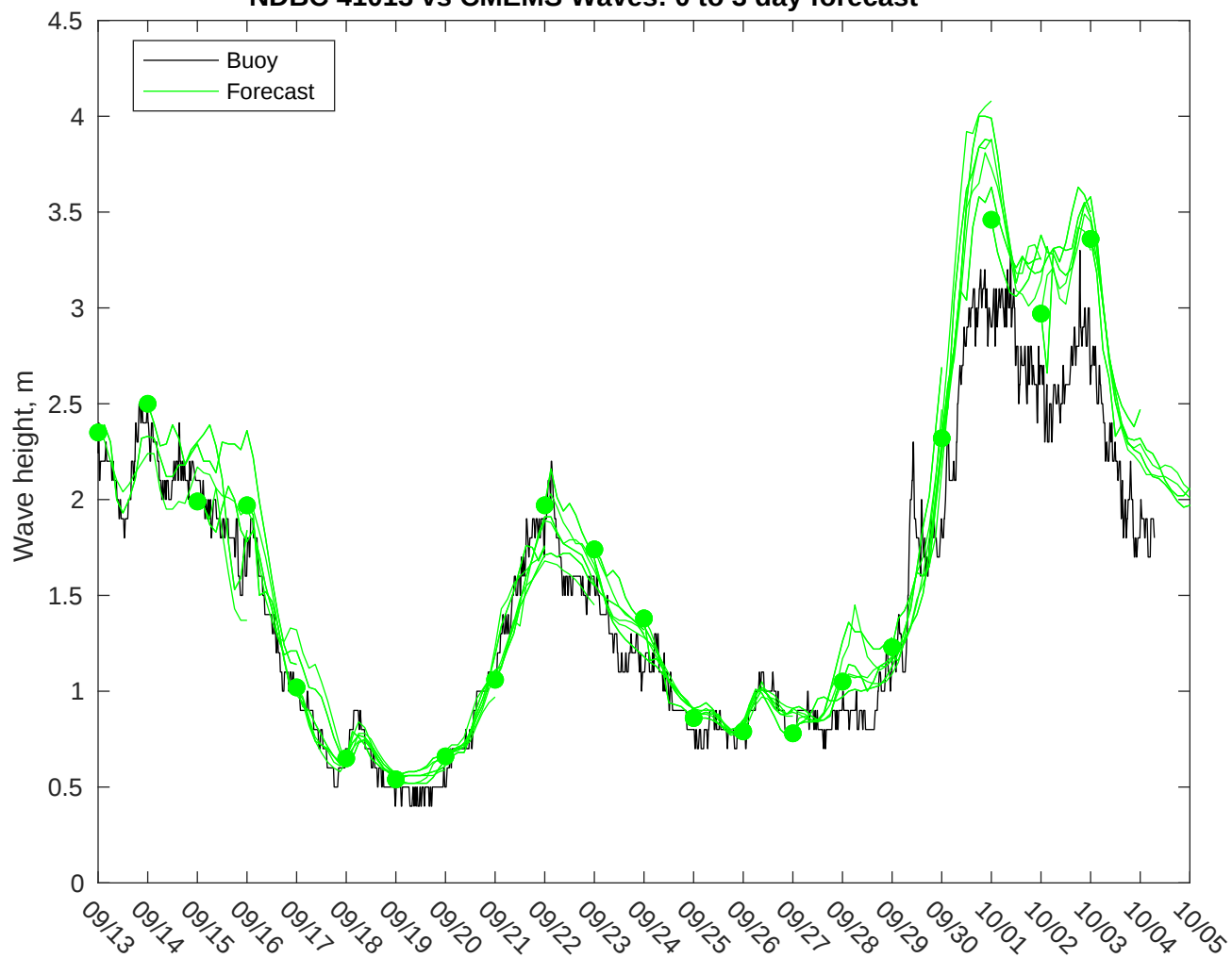
NDBC 41013 vs CMEMS Waves: 0 to 3 day forecast
