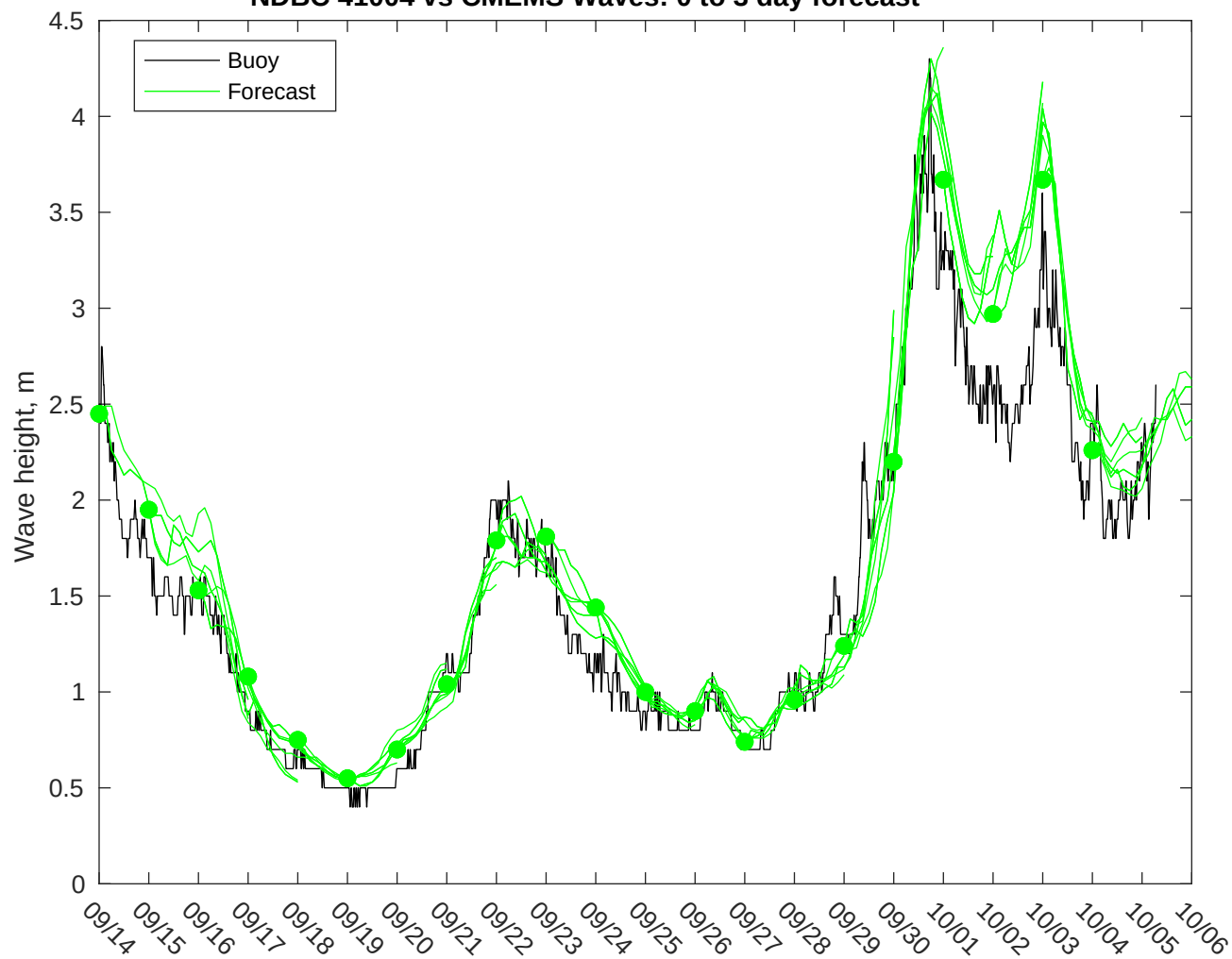
NDBC 41004 vs CMEMS Waves: 0 to 3 day forecast
