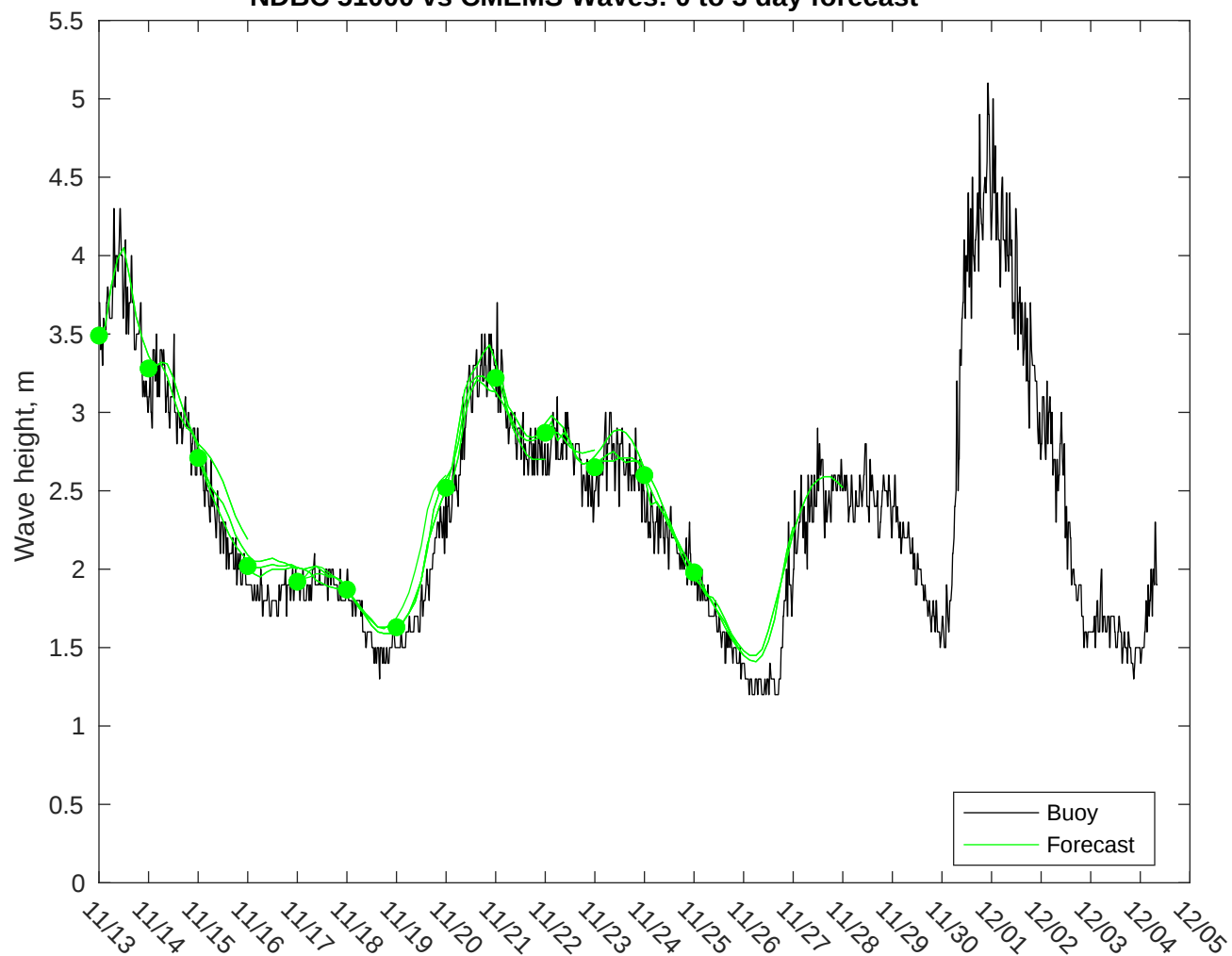
NDBC 51000 vs CMEMS Waves: 0 to 3 day forecast
