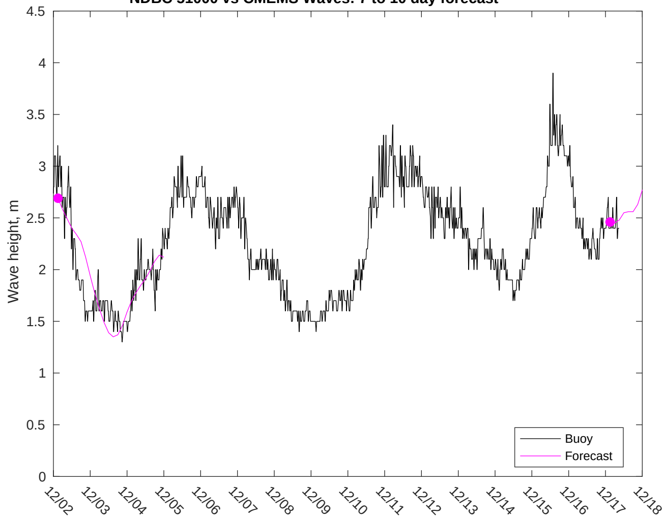
NDBC 51000 vs CMEMS Waves: 7 to 10 day forecast
