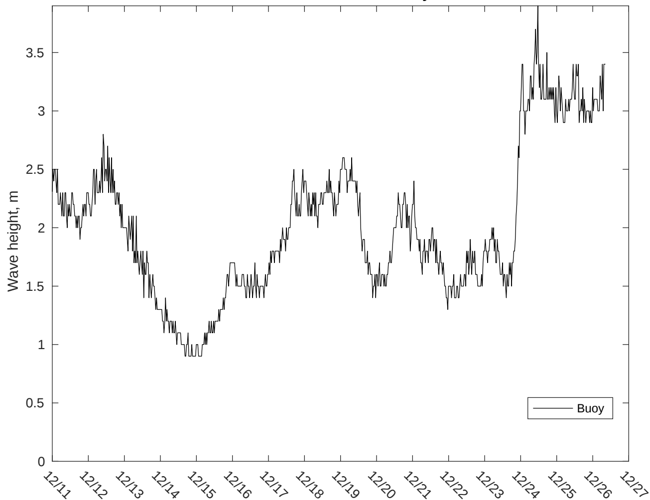
NDBC 46259 vs CMEMS Waves: 10 to 16 day forecast
