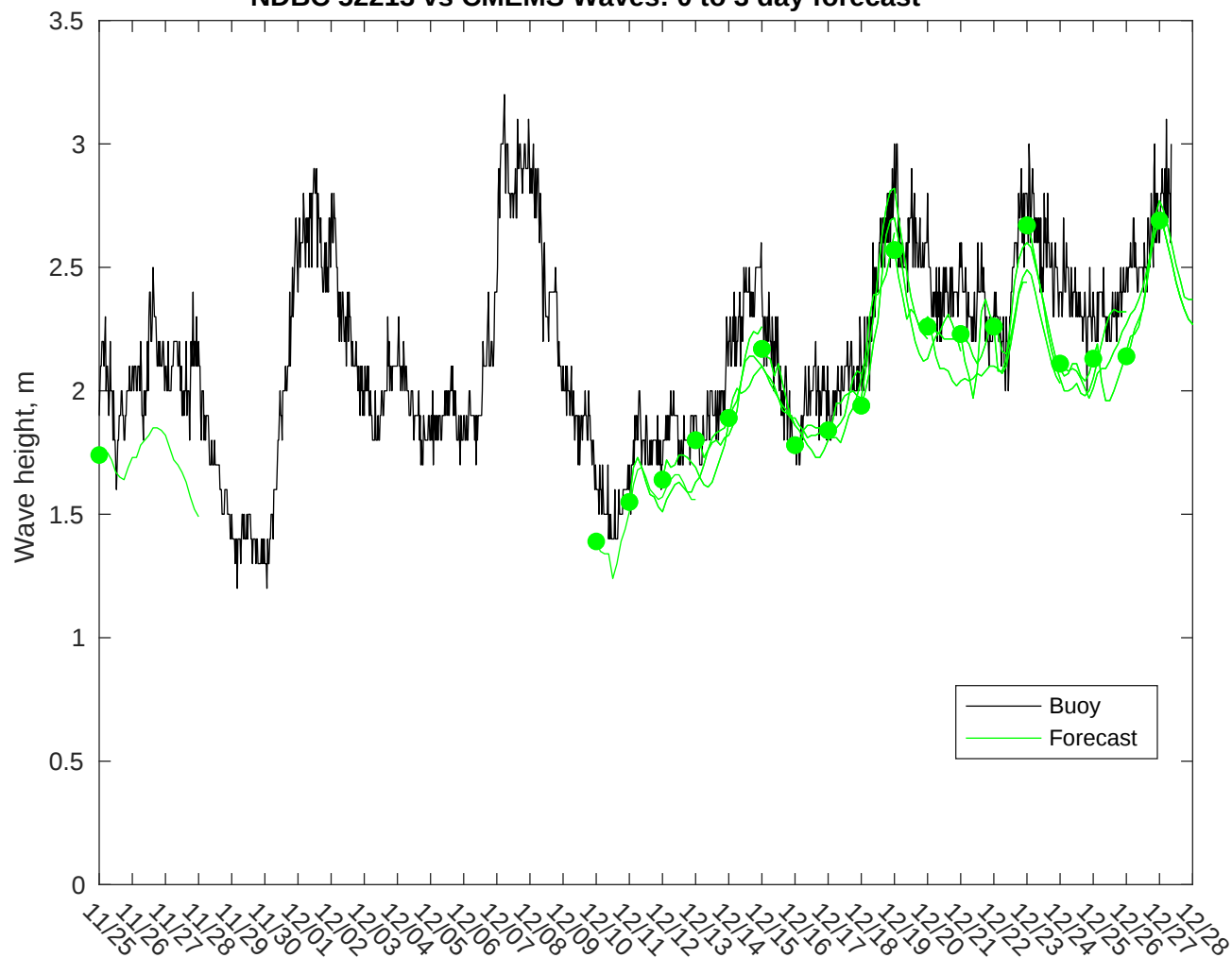
NDBC 52213 vs CMEMS Waves: 0 to 3 day forecast
