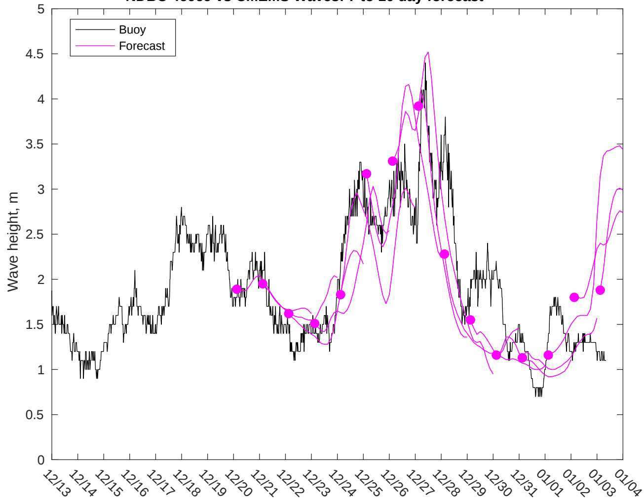
NDBC 46069 vs CMEMS Waves: 7 to 10 day forecast
