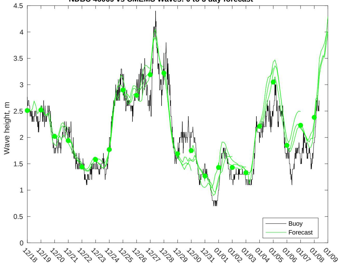
NDBC 46069 vs CMEMS Waves: 0 to 3 day forecast
