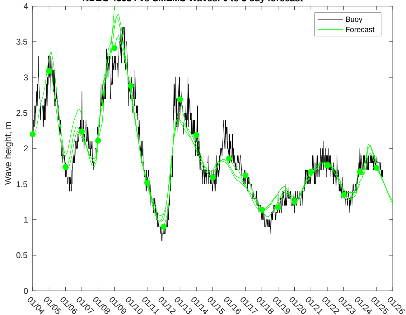
NDBC 46054 vs CMEMS Waves: 0 to 3 day forecast
