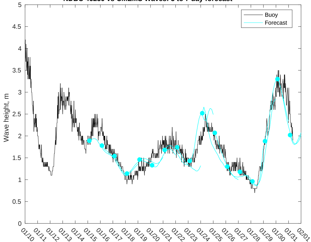
NDBC 46259 vs CMEMS Waves: 5 to 7 day forecast
